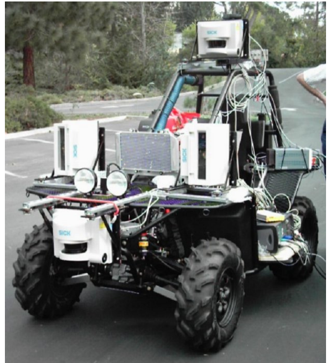
Figure 2. Lidar sensors mounted in experimental configuration with high-positioned sensor (on roof).
