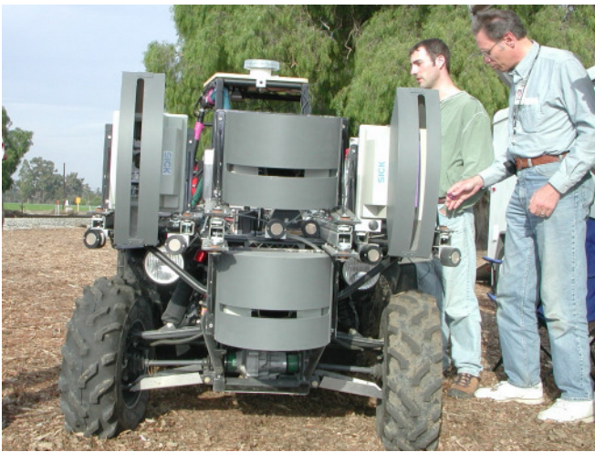
Figure 3. Shields on the Lidar to avoid perturbations.
