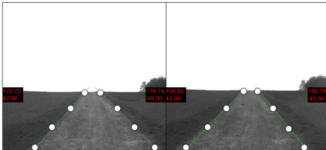
Figure 6: Results of test runs in Austria, left and right stereo image are shown. Detected lane limitations are marked and description points are shown.
