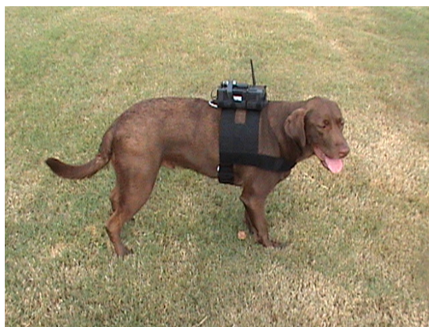
Figure 2: Canine with vest and GPS/INS system attached.
